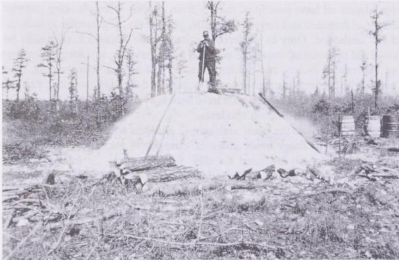
Fig. 1. Charcoal-making about 1926. Charcoal “pits” were not pits, but circular piles of wood about 4 m in diameter. Wood was stacked to a 2-m height, and then the pile was sloped toward a center stake. The surface of the piles was covered with “turf,” blocks of shrub roots, and the soil was laid with the soil side up. The pile was fired by pulling out the center stake and dropping burning kindling into the hole. The rate of burning was controlled by closing that hole and any others to produce the proper amount of draft.
