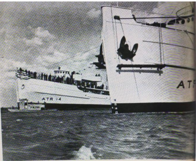
Naval Rescue Tugs Built at Leesburg on the Maurice River, New Jersey Oak Used in These Vessels.
