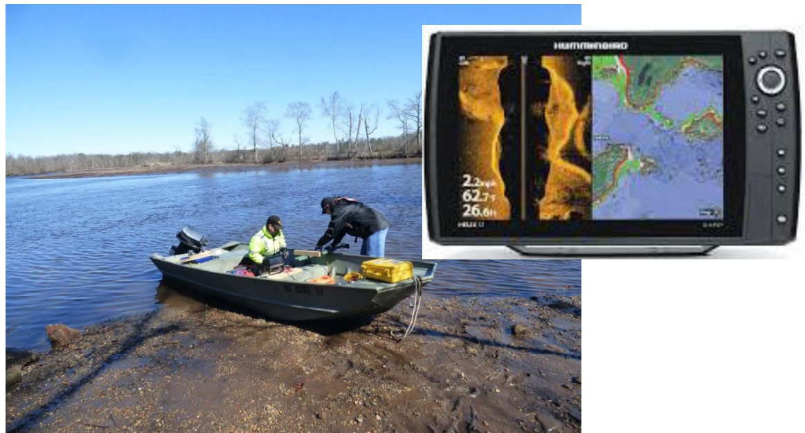
Figure 4 Stockton River Survey vessel RV Zosteria with sonar expert Vince Capone and author utilizing a Humminbird MGA 12kHz side scan sonar
